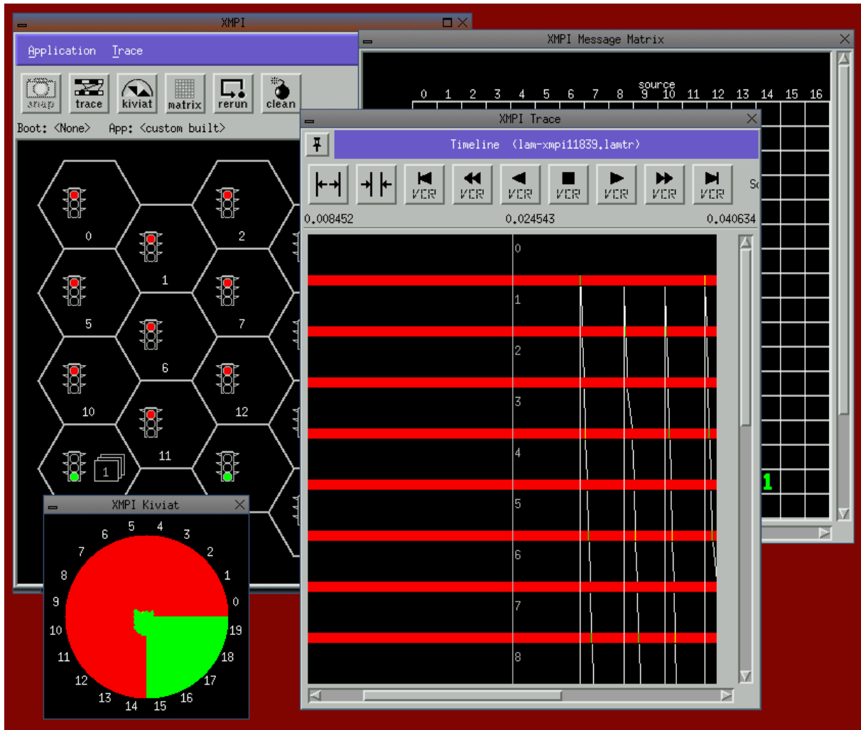
Figure 3. A LAM-MPI process as visualized through xmpi. xmpi provides graphical inspection tool to replay a parallel process. A user can visualize the sending and receiving of messages, determine the various states of the processes involved, and inspect the overall process collective's efficiency through the Kiviat tool.
