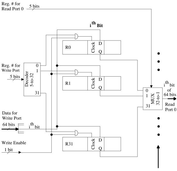
Note: To write a D flip-flop, we want its reg. # to be specified and the "Write Enable" to be asserted.
