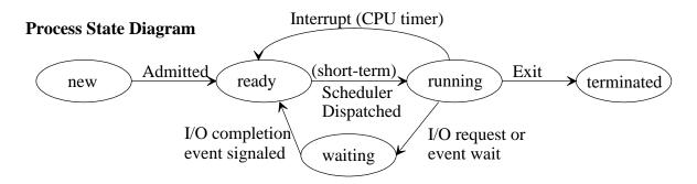
Queues are used to hold *process control blocks* (*PCB*) that represent processes internally to the OS.
