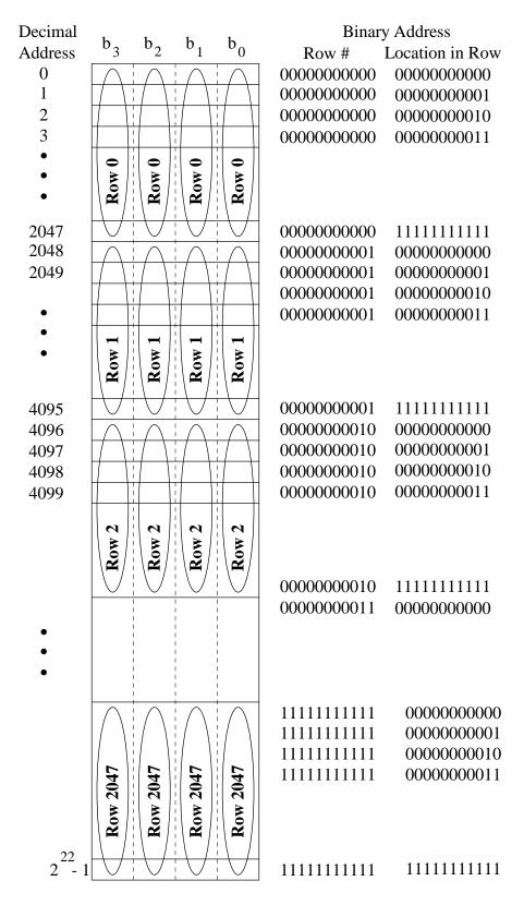
Each bit of a word is split into a separate 2048 x 2048 square memory "array". Each of these square memory arrays is  $2048 \times 2048 = 2^{11} \times 2^{11} = 2^{22} = 4M$  bits.
