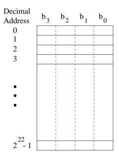
When we want to read a word, we supply a 22-bit address, and receive the corresponding 4-bit word.
