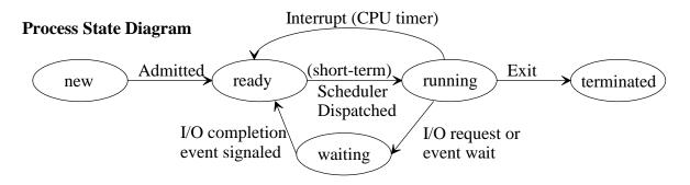
Queues are used to hold *process control blocks (PCB)* that represent processes internally to the OS.
