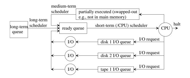
I/O queues - since I/O is so slow, several programs might have outstanding requests to use an I/O device so a queue for each I/O device is necessary.
