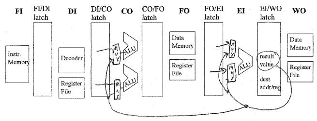
a) For the six stage pipeline of the text (see above), complete the following timing diagram assuming NO by-pass signal paths. (RECALL that LOAD reads a memory value into a register; STORE saves a register to memory) Assume that we cannot write to a register and read from that same register in the same clock cycle.
