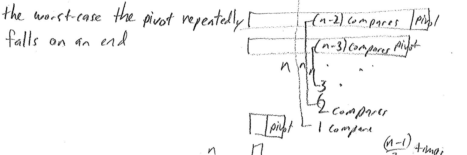
$$\# \text{ compares} = (n-1) + (n-2) + (n-3) + \dots + 3 + 2 + 1 = \underbrace{n + n + \dots + n}_{\frac{(n-1)}{2} + 1 \text{ terms}} = n \times \frac{(n-1)}{2} \in O(n^2)$$
