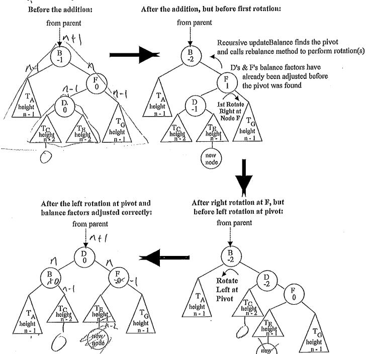
b) Suppose that the new node was added in Tc instead of T<sub>B</sub>, then the same two rotations would restore the AVL-tree's height-balance property. However, what should the balance factors of nodes B, D, and F be after the rotations?
