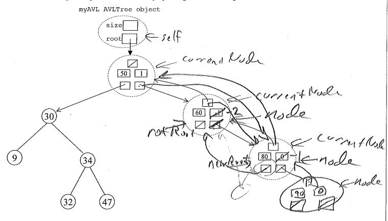
Consider balance factor formulas for rotateLeft. We know:  $newBal(B) = h_A - h_C$  and  $oldBal(B) = h_A - (1 + max(h_C, h_E))$  $newBal(D) \neq 1 + max(h_A, h_C) - h_E$  and  $oldBal(D) = h_C - h_E$
