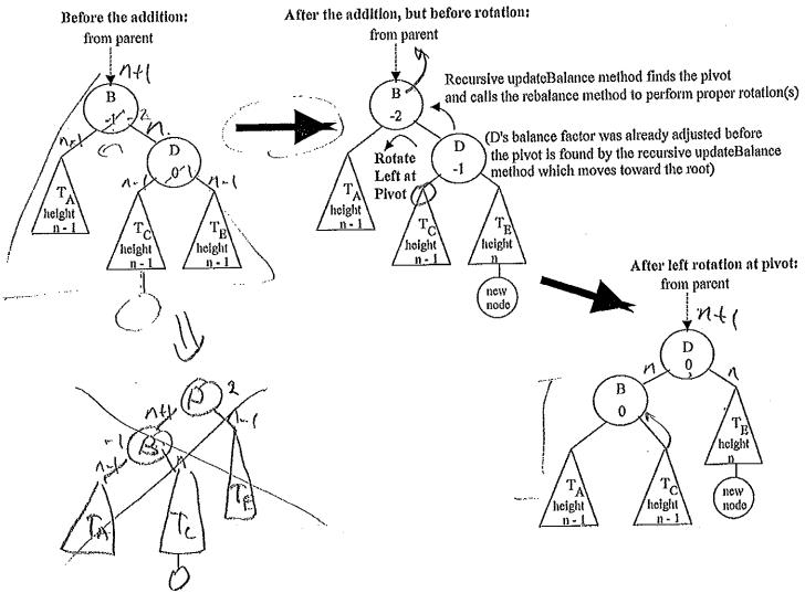
a) Assuming the same initial AVL tree (upper, left-hand of above diagram) if the new node would have increased the height of  $T_c$  (instead of  $T_E$ ), would a left rotation about the node B have rebalanced the AVL tree?
