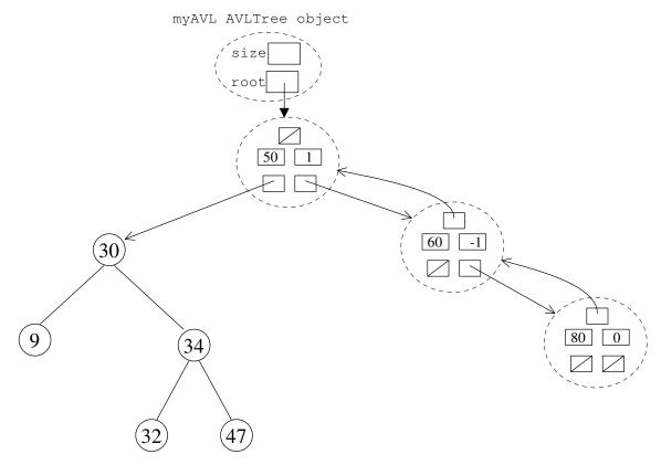
Consider balance factor formulas for rotateLeft. We know:  $newBal(B) = h_A - h_C$  and  $oldBal(B) = h_A - (1 + max(h_C, h_E))$
