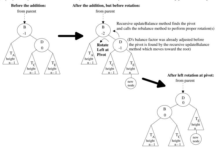
a) Assuming the same initial AVL tree (upper, left-hand of above diagram) if the new node would have increased the height of  $T_c$  (instead of  $T_e$ ), would a left rotation about the node B have rebalanced the AVL tree?
