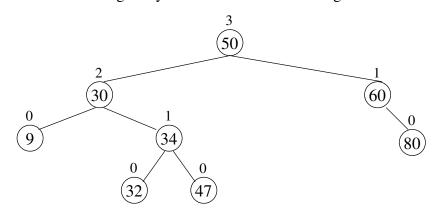
Each AVL-tree node usually stores a *balance factor* in addition to its key and payload. The balance factor keeps track of the relative height difference between its left and right subtrees, i.e., height(left subtree) - height(right subtree).
