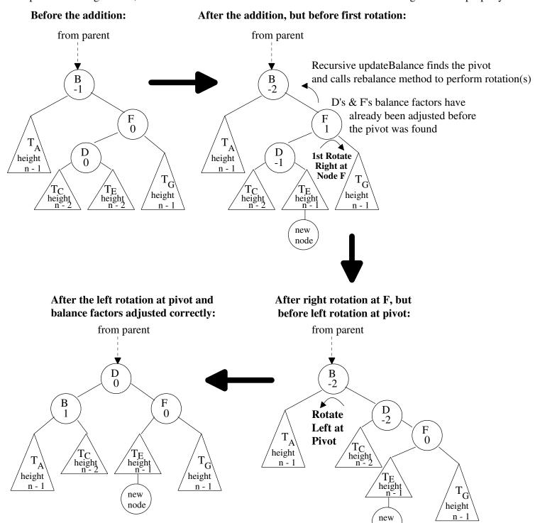
b) Suppose that the new node was added in  $T_C$  instead of  $T_E$ , then the same two rotations would restore the AVL-tree's height-balance property. However, what should the balance factors of nodes B, D, and F be after the rotations?
