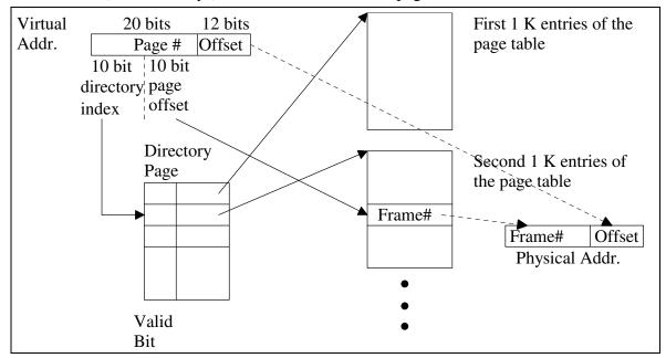
A 64-bit computer might not support a full 64-bit address space. How could a 3-level page table support 42-bit address space?
