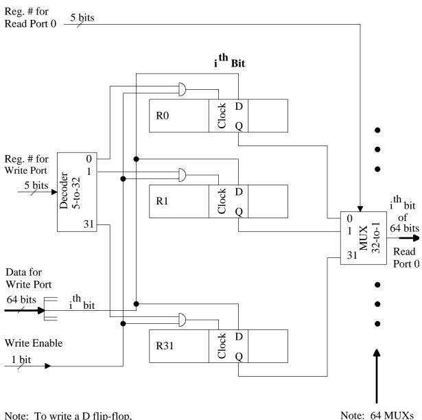
Note: To write a D flip-flop, we want its reg. # to be specified and the "Write Enable" to be asserted.
