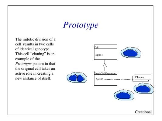
The *Prototype* pattern specifies the kind of objects to instantiate using a prototypical instance.
