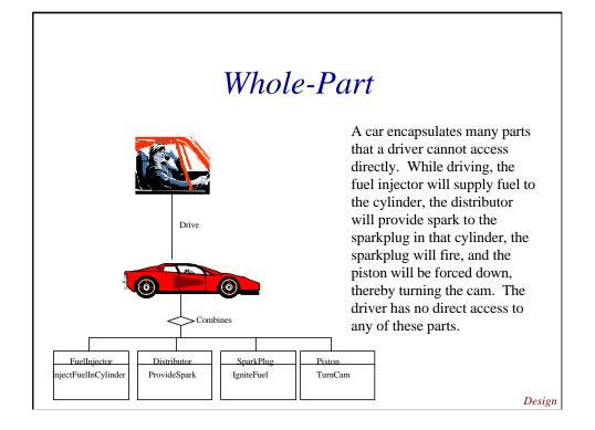
The Whole-Part pattern helps aggregate components that form a semantic unit.
