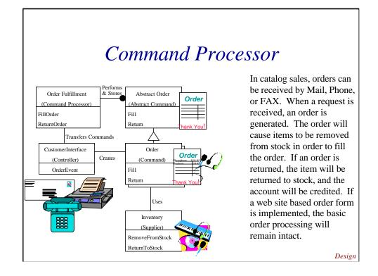
The *Command Processor* pattern separates the request for a service from its execution.
