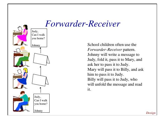
The *Forwarder-Receiver* pattern introduces a peer-to-peer communication model that decouples the forwarders and receivers from the underlying communication mechanisms.
