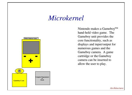
The *Microkernel* pattern separates the minimal functional core from extended functionality.
