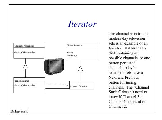
The *Iterator* provides ways to access elements of an aggregate object sequentially without exposing the underlying structure of the object.
