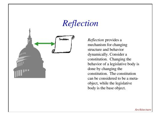
The *Reflection* pattern provides a mechanism for changing structure and behavior of a system dynamically. A system is structured as a base level, and meta level. The meta level contains information about system properties. The base level exhibits the application structure and behavior. Changes to meta level information affect subsequent base level structure and behavior.
