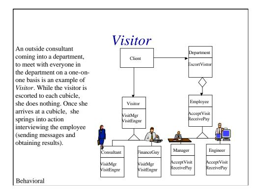
The *Visitor* pattern represents an operation to be performed on the elements of an object structure, without changing the classes on which is operates.
