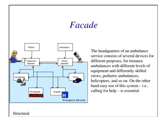
The *Facade* defines a unified, higher level interface to a subsystem, that makes it easier to use.
