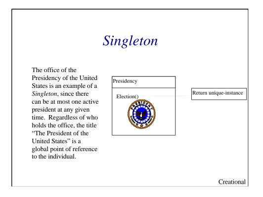
The *Singleton* pattern ensures that a class has only one instance, and provides a global point of reference to that instance.
