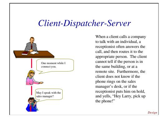
The *Client-Dispatcher-Sever* introduces an intermediate layer between clients and servers to provide location transparency and hide connection details.
