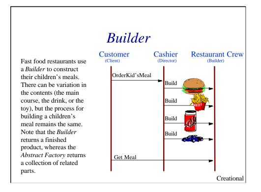
The *Builder* pattern separates the construction of a complex object from its representation, so the same construction process can create different representations.
