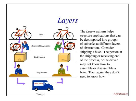
The purpose of *Layers* is to structure applications that can be decomposed into different subtasks, with each subtask at an appropriate level of abstraction.
