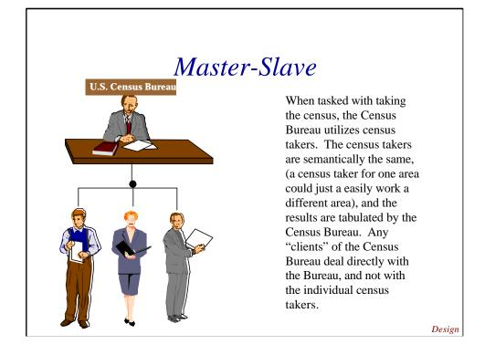
A master component distributes work to identical slave components and computes a final result from the results when the slaves return
