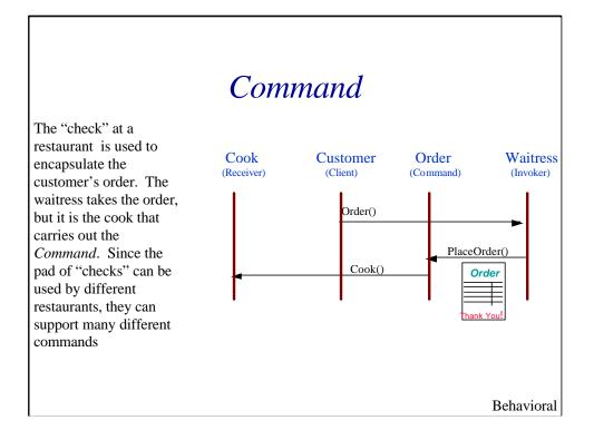
The *Command* pattern allows requests to be encapsulated as objects, thereby allowing clients to be parameterized with different requests.
